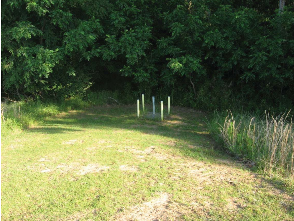
Groundwater Monitoring Well on North Toe of Dam
