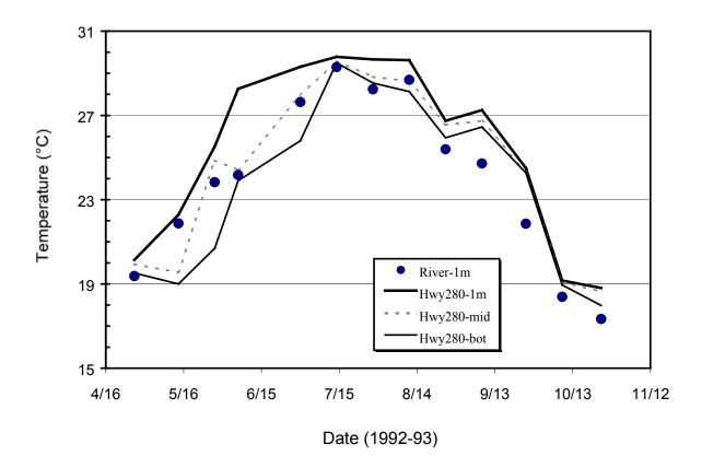
**Figure 3**. Temperature at Hwy 280 by depth and date for April to October 1992. The plot also shows the temperature at 1 m for the Flint River as it enters Lake Blackshear at GA 27.
