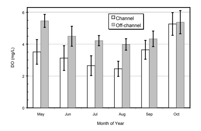
**Figure 5**. Comparison of monthly mean near-bottom DO concentration at channel and shallow offchannel sampling sites in Lake Blackshear from 1997 to 2001. Data were collected by Weyerhaeuser Mill staff.
